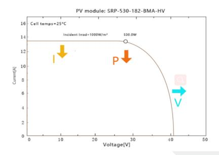
Power decline happens very often during middays, and always occurs before current decline, research shows DC losses due to current decline will have subtle difference when the DC/AC ratio is higher than 1.25. Therefore, there is no yield loss due to current decline when the DC/AC ratio is larger than 1.25 in Australia.
