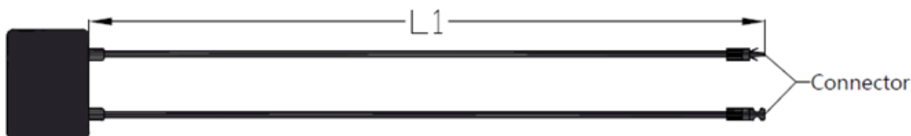
Figure 11 (1): The full module junction box
